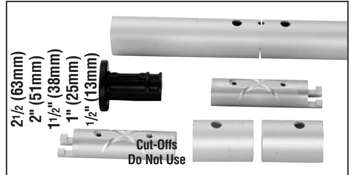
2 1/2" - 1/2" (63 - 13mm) Shorten top foil and adjoining full length foil so two screws are used to assemble joint instead of four. Do not use plastic bushings above top connector.
